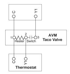
Figure 22: Taco SBV Valve Wiring
